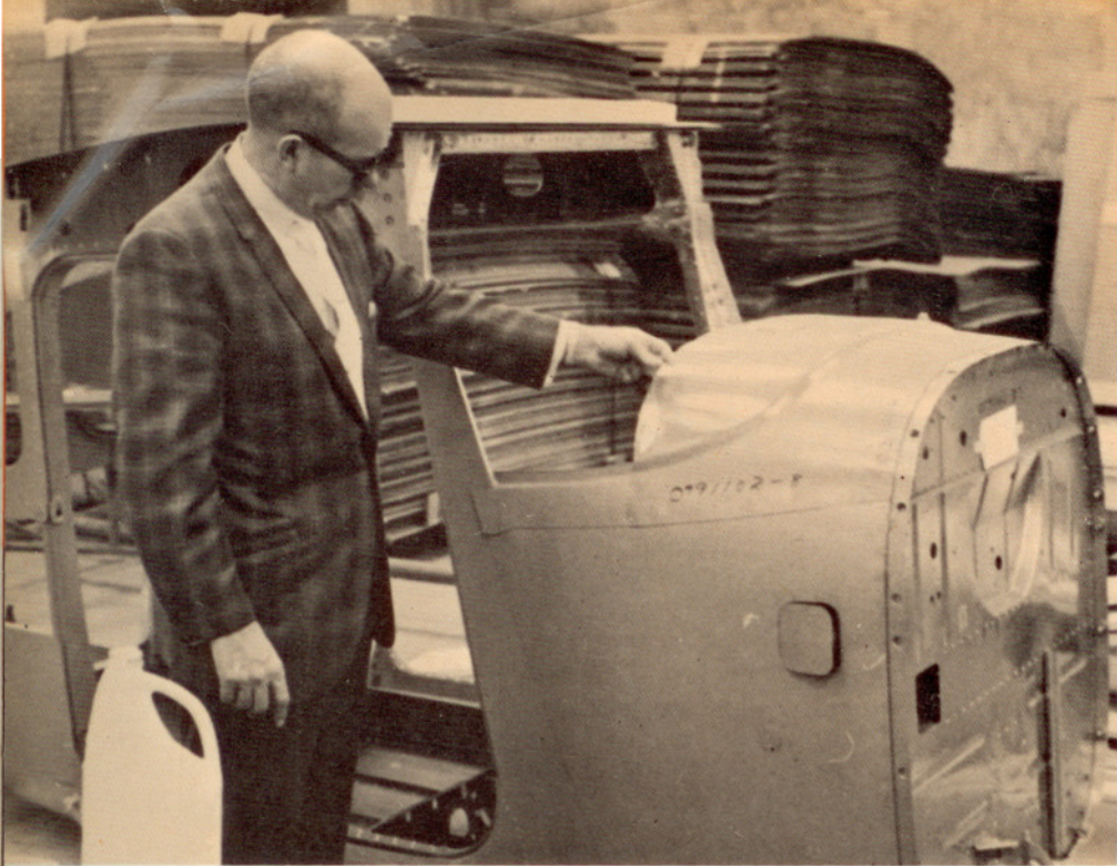
Cessna Customer Services Director L. C. Gartin inspects a plastic-like substance sprayed on a cabin section for protection during shipment to Green River Aviation, Ogden, Ut. The order was received at the factory Dec. 10 and was being readied for shipment Dec. 16.
